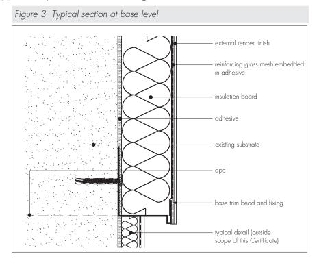
16.6 The insulation board adhesive is prepared using Powerwall Adhesive Coat powder, which is mixed for at least five minutes with water using an electric paddle mixer. One litre of water is used with 4.5 kg of powder. The adhesive is applied to the complete surface of the insulation board using a notched trowel before securing the insulation board to the wall (see Figure 4).
